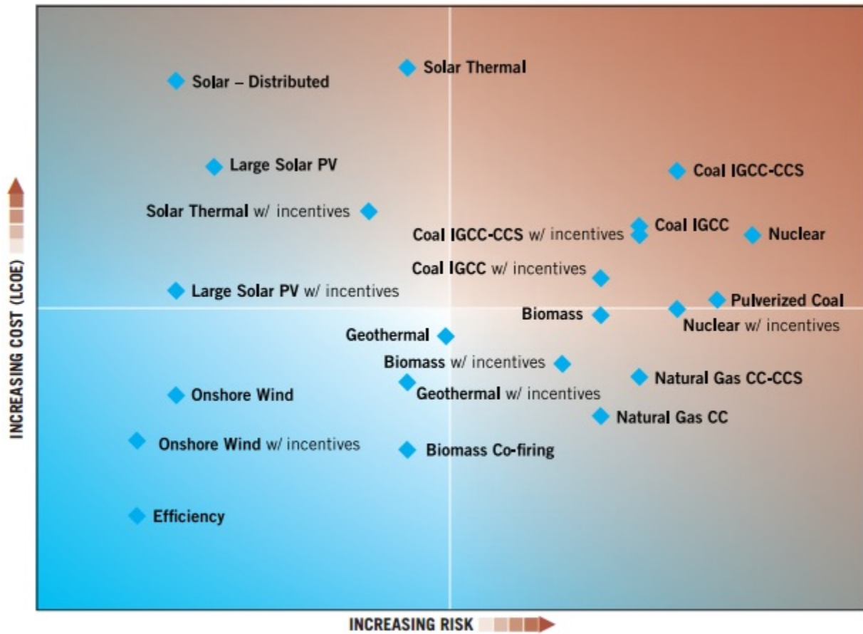
Figure 26. Relative cost and risk of utility generation resources
